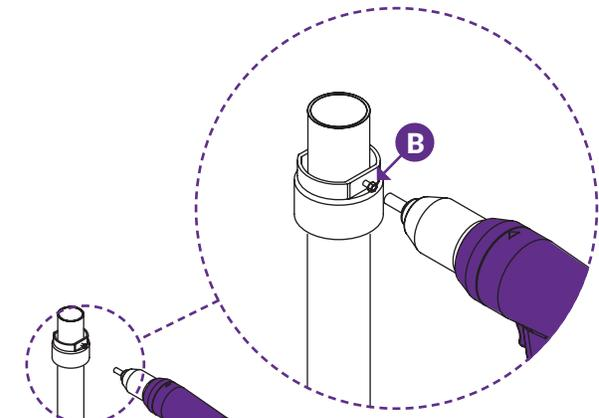
*Note: The donut can be adjusted to compensate for a slightly crooked pipe anchor. Slide the donut either left or right to create a level plane between the anchor positioner and the donut.*
